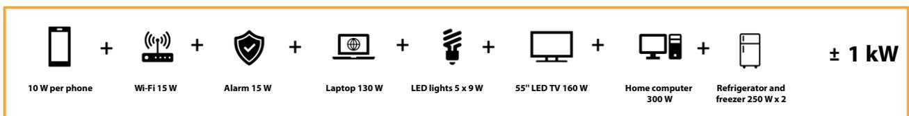
Remember that not all appliances are switched on the whole time or simultaneously, but – in the worst case – take the total load as 1 kW to determine how much energy to store.
