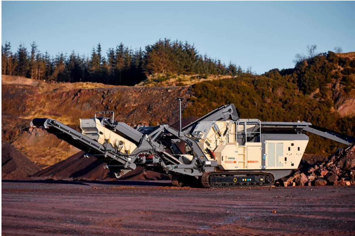
Caption: Metso Nordtrack™ 1908S mobile impactor plant – part of the new mobile Nordtrack™ crushing and screening product range for the aggregates industry.
