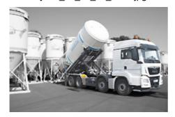
The ZTA is a device for silos ranging from 12 m³ to 22 m³ loading volume for the 2-pocket silo system, which is widely used on the market.
