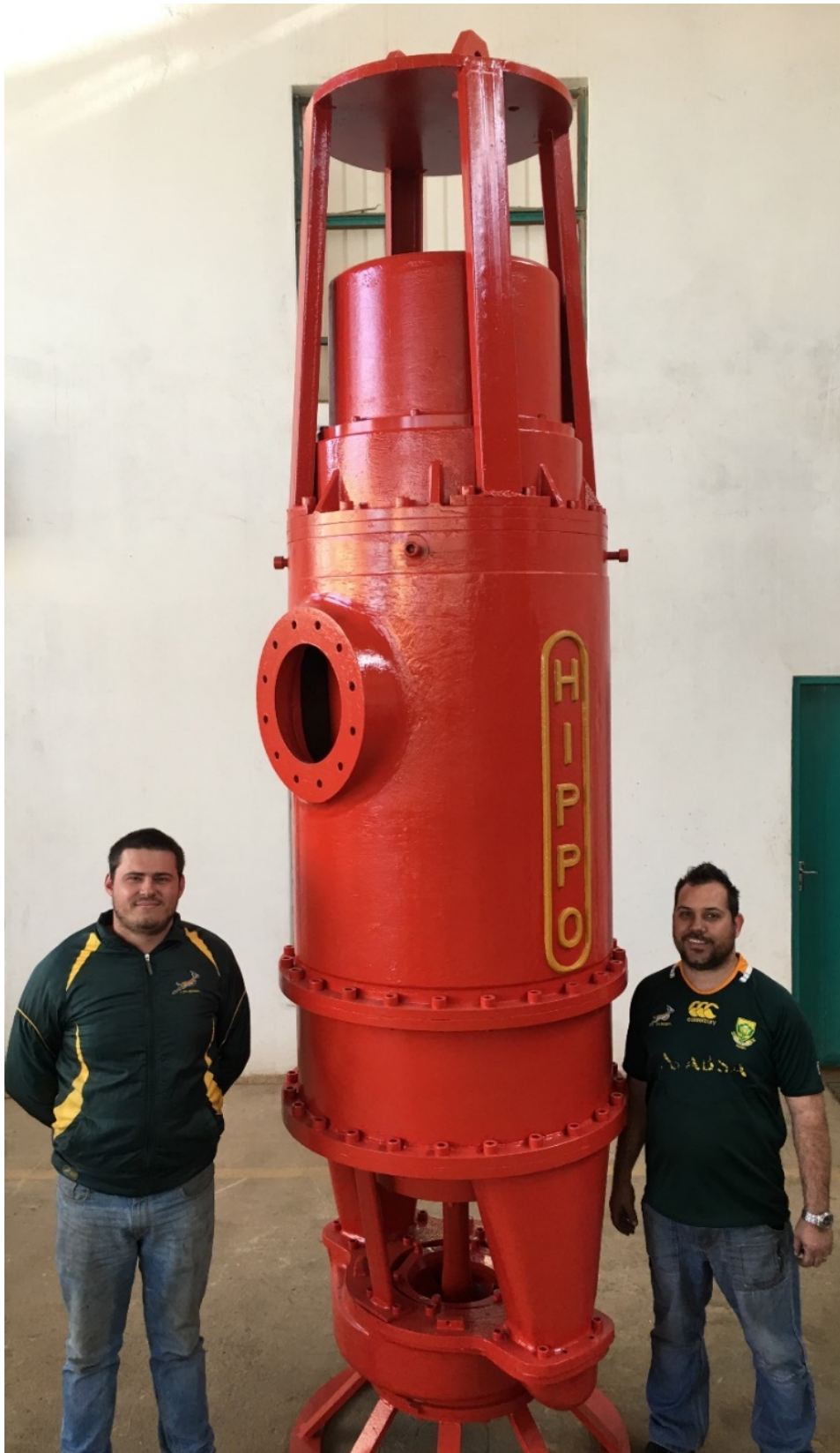
The only Medium/High Voltage; High Head; High Volume; Flameproof Submersible Slurry pump in the world pumping heads of 250 meter at the best efficiency point.
