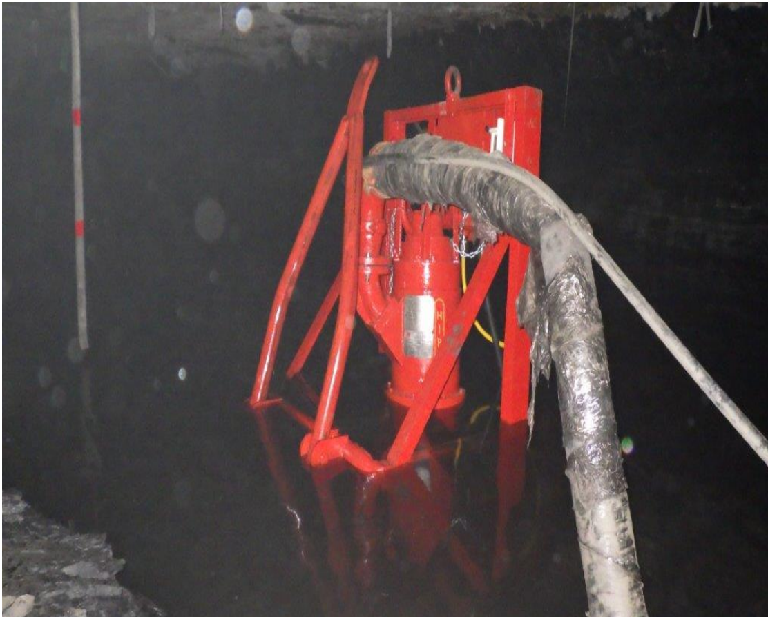
The skid mounted HIPPO Flameproof Submersible Slurry Pump System® in underground operation in a typical coal mine
