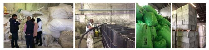
FLTR: Sedick Samsodien explains to the guests attending the factory tour how the mountains of post-consumer and post-recycled polystyrene visible in the background are collected and recycled into the Greenlite lightweight concrete bricks and screed used to build shopping malls, architectural homes and low-cost housing.
