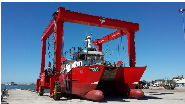
The boat hoist brings a vessel ashore.
