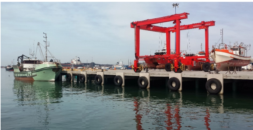
The 90 ton boat hoist in action.
