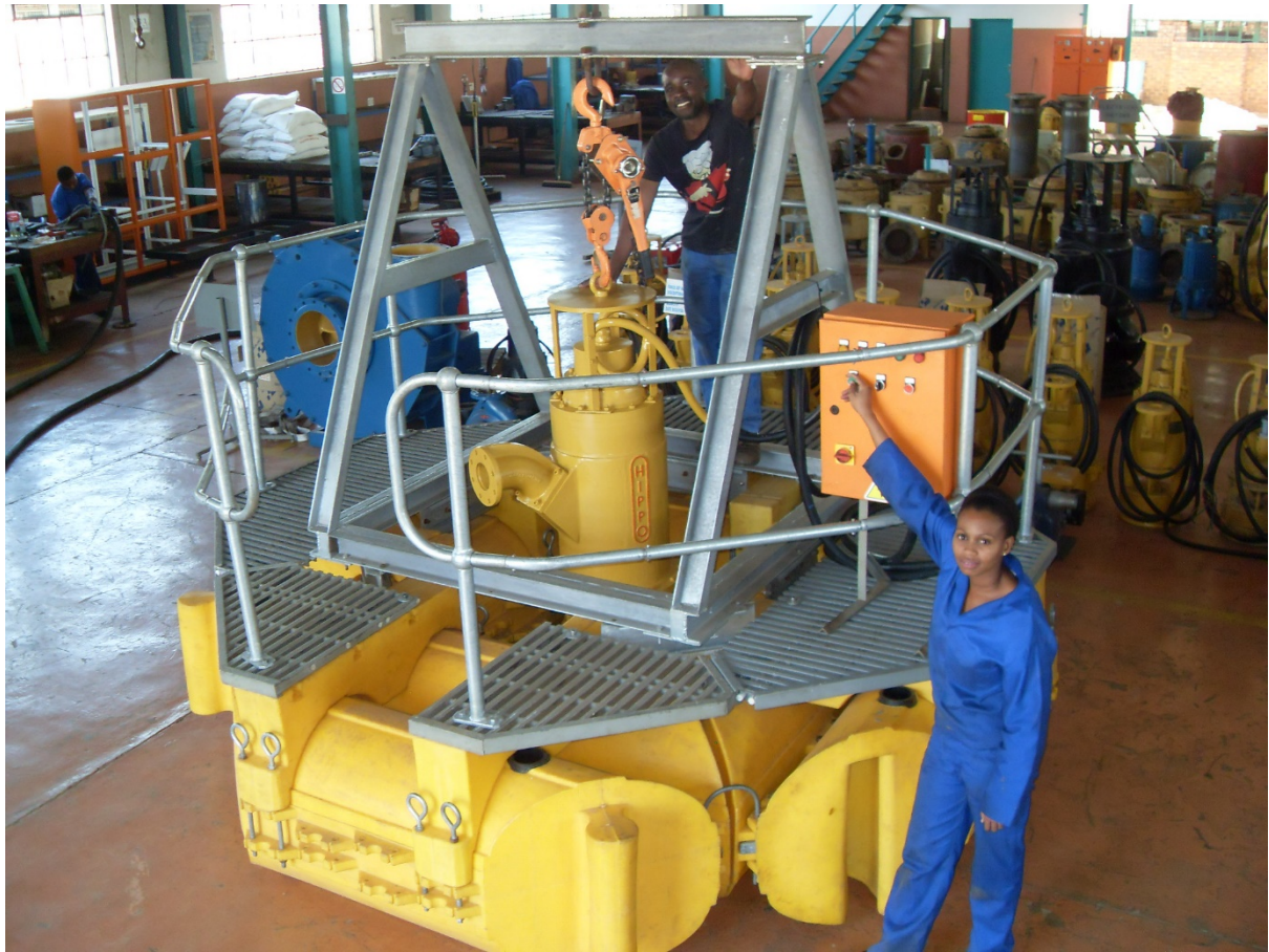
HIPPO Submersible Slurry Pump® mounted on pontoon complete with electrical switchgear and lifting equipment
