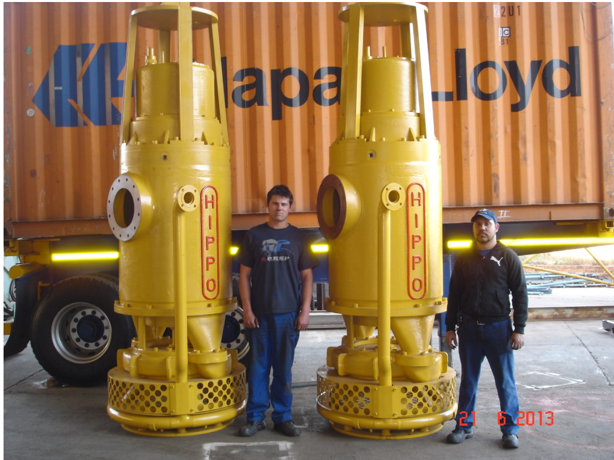
The first two HIPPO submersible slurry pumps that were designed, developed and manufactured in South Africa to be exported to the oil sands mines in Canada
