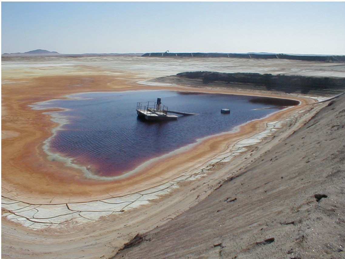
A HIPPO vertical spindle pump mounted on a pontoon in operation at the Rössing Uranium mine in Namibia
