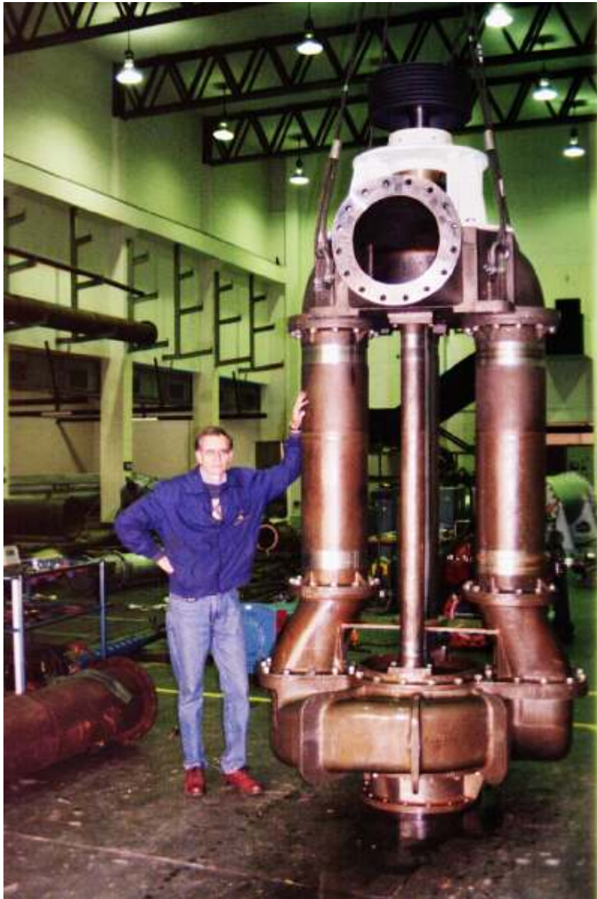
The HIPPO model 400 VNB vertical spindle pump manufactured From a Nickel alloy to handle phosphoric acids
