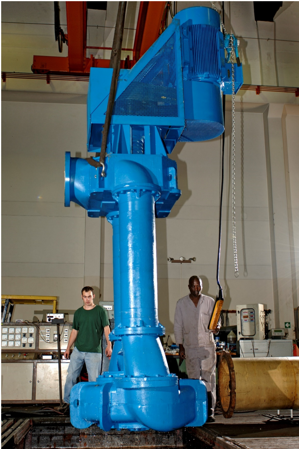
The largest vertical spindle froth slurry pump in the world designed and manufactured in South Africa for a phosphate plant in Russia
