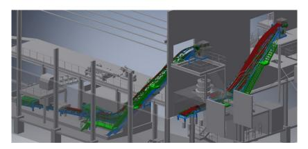
The DSI Sandwich high angle conveyors will serve as transfer conveyors elevating crushed pebble ore, each at a rate of 135 t/h and a 45° incline for Continental Gold's Buriticá project in Antioquia, Columbia.
