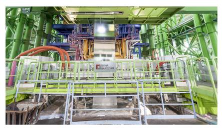
In the future, a DUMA-BANDZINK Jet-Pro air knife system will produce high-quality surfaces in the hot-dip galvanizing line No. 3 of SSAB, Finland. (The picture shows a plant of similar design).
