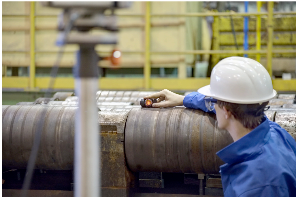
Reliable measurement of continuous caster segments and molds using the HD LASr plant assistant system from SMS group.
