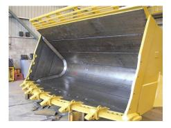
The smooth, dense metal alloy face and hard steel back plate resist gouging, erosion and extreme temperatures.
