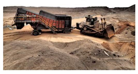
The concept of the Samson® Material Feeder was developed to satisfy the demands of clients requiring a mobile solution to receive general bulk materials such as coal and aggregates direct from tipping trucks where fixed plant was not a viable option.
