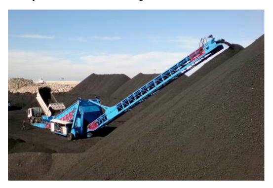
A unique concept in Bulk Materials Handling, the Stormajor® combines the benefits of the Samson® Material Feeder design with a radial and luffing outloading boom conveyor into a single mobile machine able to receive material both from tipping trucks and loading shovels.
