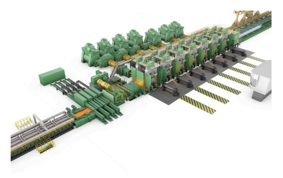
At Nucor Steel Berkeley, the new modernization concept with inductive heating systems between CSP<sup>®</sup> furnace and CSP<sup>®</sup> rolling mill was implemented for the first time.
