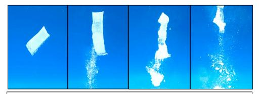
After immersion EcoSol® dissolves in water leaving a harmless, non-toxic, aqueous solution of polyvinyl alcohol. Microorganisms will degrade the solution to carbon dioxide and water within about 30 days.
