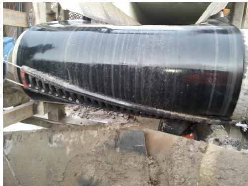
CleanScrape forms a three-dimensional curve beneath the discharge area that conforms to the pulley's shape.
