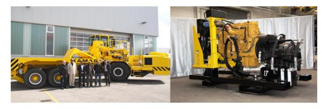
The current generation of the KAMAG scrap basket transporter for the Saudi Arabian steel giant, Hadeed has an innovative surprise under the bonnet: the modular drive unit can be easily removed for maintenance purposes. This results in enormous time savings compared to conventional designs and therefore dramatically reduces the downtime.
