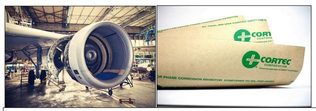
VpCI® 146 was used for preservation of Indian Navy's Naval Aircraft Engine. After inserting Cortec's VpCI®132 Foam Pads, the entire engine was wrapped with VpCI®146 paper and sealed. By switching to Cortec's method, the navy saved 60 - 70% on current costs and gained a non-hazardous, environmentally friendly solution for long term storage.
