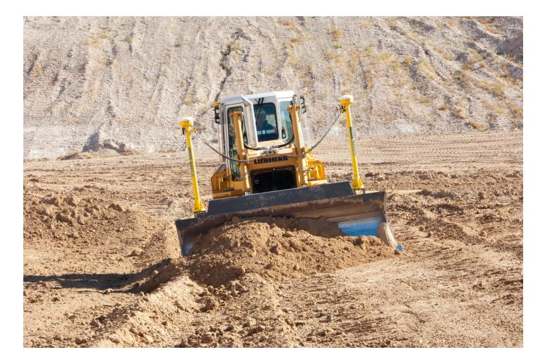
GCS900 version 12.7 features GradeMax<sup>™</sup> Plus, new technology that increases the overall performance of dozers by allowing the operator to grade faster and more consistently with tighter accuracy. GradeMax Plus technology allows contractors to grade between 35 and 40 percent faster on average, depending on the dozer type and the material being used.
