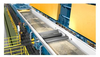
The turbulence pickling line achieves optimum descaling results with low consumption of energy and pickling liquor, while keeping maintenance and operating costs low.
