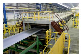
The new line will be used to pickle 1.3 million tons per year of hot strip as a preparation for its future application in the building sector.
