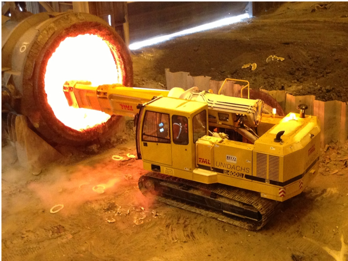
TML's Unidachs hot ladle machine in action
