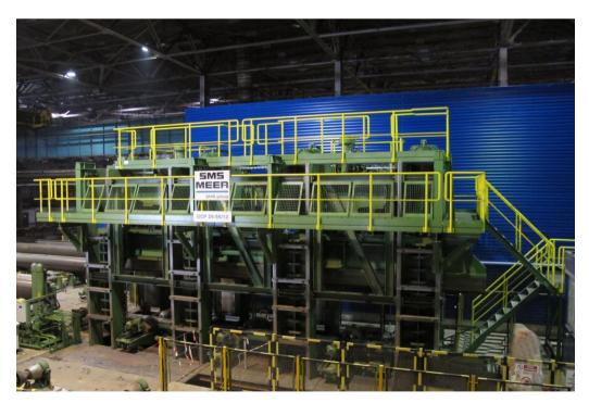
Thanks to the variable-speed pump control VSP, the machine consumes 50 percent less energy than the older machine generation.
