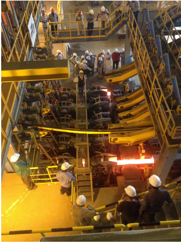
The first cast in the continuous caster was successful.
